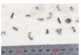
Remaining pip in the centre : \phi 1.42 mm RZ : 0.015 mm
