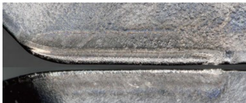
5.0m cutting length achieved MV1020
