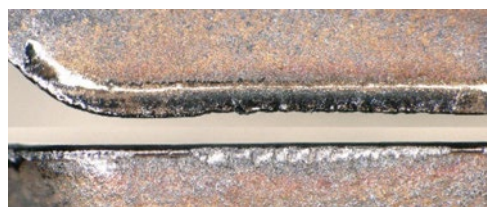
Wear progressed and the substrate was exposed
