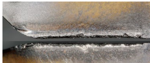
Chipping occurred due to peeling of the coating Conventional
