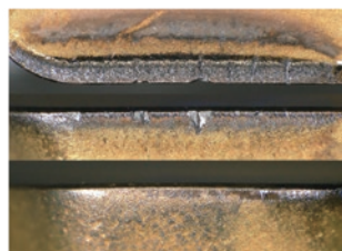
Chipping occurred due to thermal cracks at a cutting length of 2m
